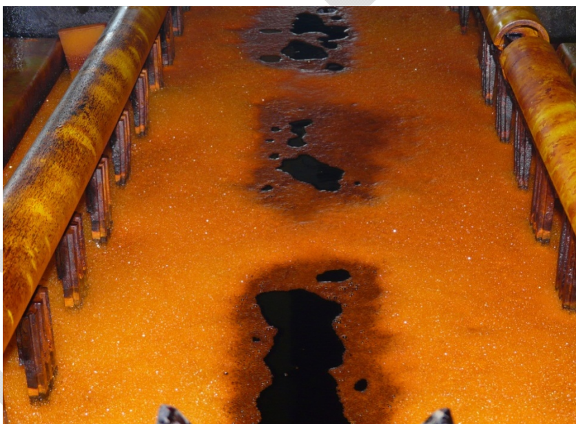
Figure 4-1: Foamy barrier on the surface of a chromium bath
